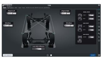
Cross-diagonal measurements to determine accident damages
